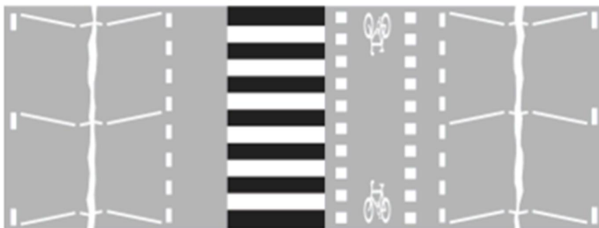
Figure 8-3: Parallel crossing to make provision for cyclists
